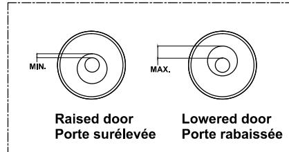
**\*\* Rotate this accessory with wrench to adjust rollers up and down, let the door glass in a horizontal state.**
