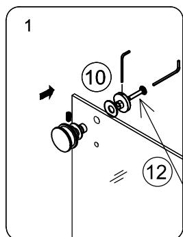
**\*\*Apply "Loctite" glue on the thread of the Rollers' screw before the installation.**
